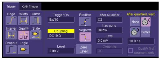
The "Trigger On" condition is that of the normal pulse output from the CAN Trigger module, and the Qualifier is your analog signal.
