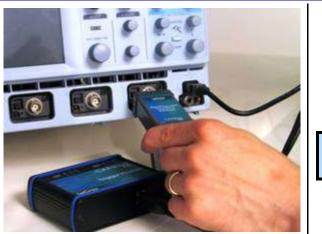
Connect the CANbus TD/TDM Oscilloscope Interface Module (OIM) to the EXT input of the instrument. Make sure that the top (OIM labeled side) is facing up.
