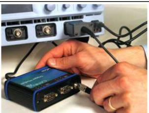
4. Connect the 3-pin plug end of the OIM to the Trigger Module.
