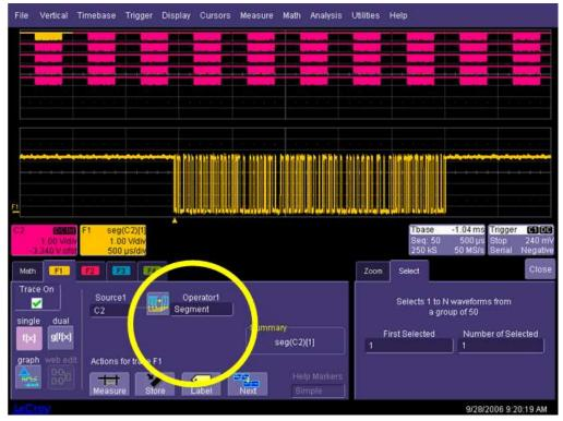
7. Set up the Decode to use the Math trace as the source for Data in order to view decoded data on the individual segment (in this case F4 is the source).
