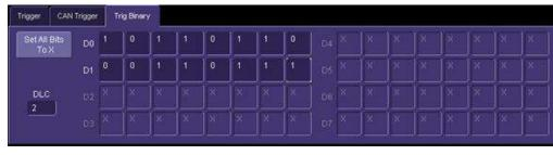
The Data Bytes are labeled D0 through D7. The far left bit in each byte is bit 7 and the far right bit is bit 0. A "1" is always a dominant bit, and a "0" is always a recessive bit. An "X" means that the bit can be either a 1 or a 0. Select a bit value by touching the existing value and choosing a value from the pop-up menu. The data bytes shown in the Binary trigger setup dialog are always in LSB (Least Significant Byte) format.
