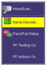
3. **Decode Protocol Selections** - CAN is one of several signal types that can be decoded by the oscilloscope. Other standards include I2C, SPI, UART, RS-232, LIN, and FlexRay.
