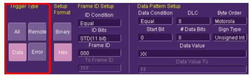
• All - Triggers on all signals. No Frame ID and Data Pattern ID Setup fields are enabled.
