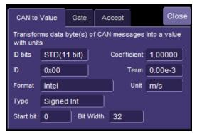
You must specify the ID length and ID Value for the CAN Messages that you wish to extract data from. The measurement parameter will process all messages meeting the ID condition in the acquisition, and apply the same conversion to them.
