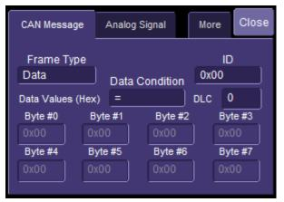
The CAN Message tab defines the CAN Message Setup. The Analog Signal tab defines the Analog Signal Setup.
