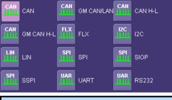
**Note**: SIOP and SSPI are part of the SPIbus TD package. RS232 is part of the UART-RS232bus TD package.
