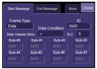
The Start Message tab defines the first CAN Message Setup. The End Message tab defines the second CAN Message Setup.
